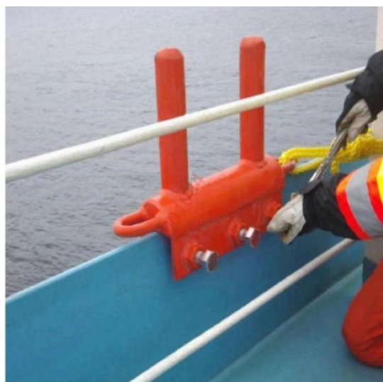
Figure 4.1.1(2) Portable chock used to deploy secondary fender pennant
