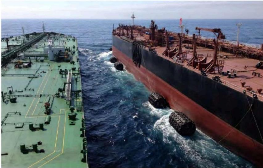
Figure 5.4 Berthing should not commence before establishing communication contact.
